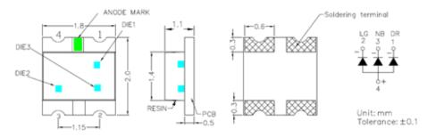
1. Soldering terminal may shift in x, y direction.
